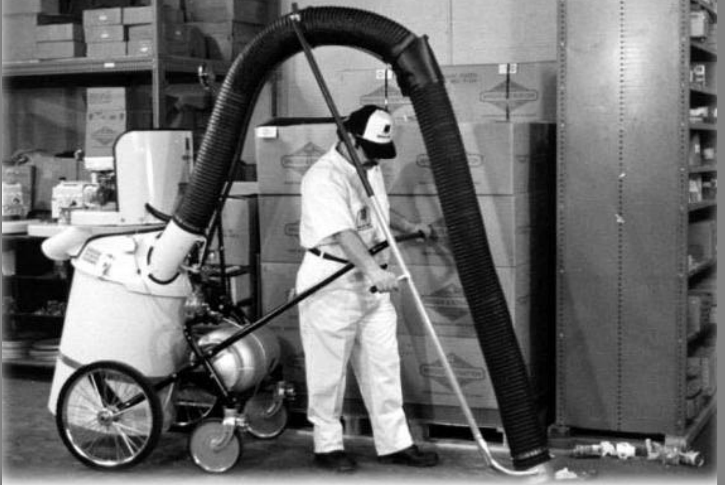
Elephant-Vac model 650-IP LP gas powered vacuum.
